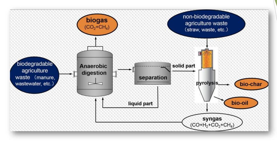
The proposed processing plant for the conversion of both biodegradable and non-biodegradable agricultural residues into useful bio-products and/or hydrogen feeding SOFCs for energy production
